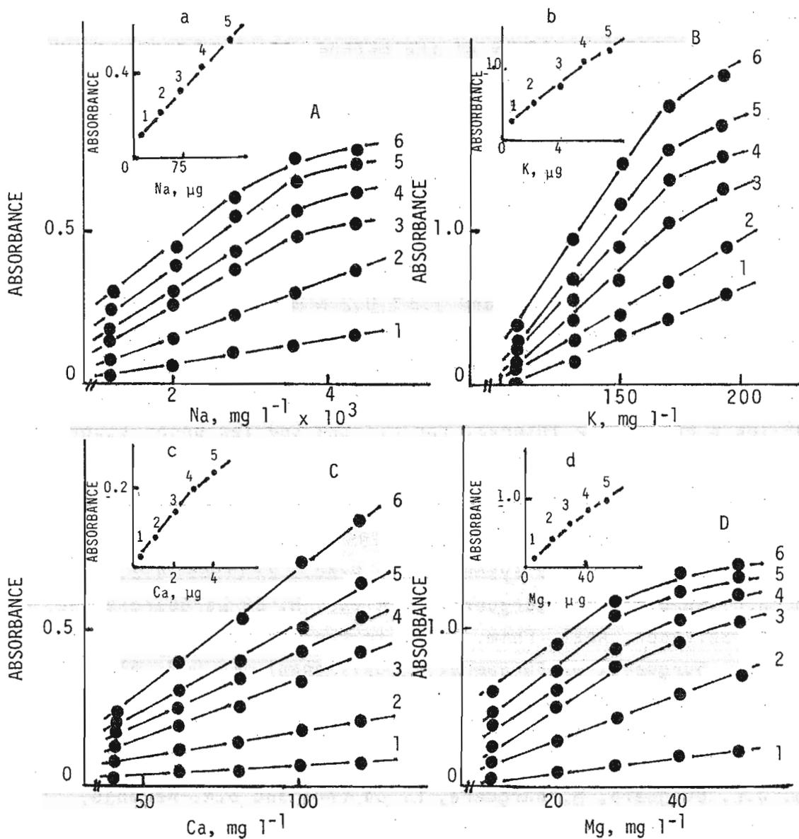
Fig. 4 A-D: Variation in peak height with sample volume. 1 to 6 indicate the sample volumes 4, 14, 22, 34, 48 and 62  $\mu$ l, respectively.
