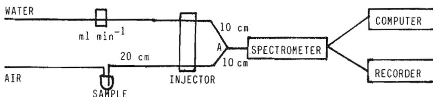
Fig. 1 Flow diagram for the determination of sodium, potassium, calcium and magnesium using the variable volume injector
