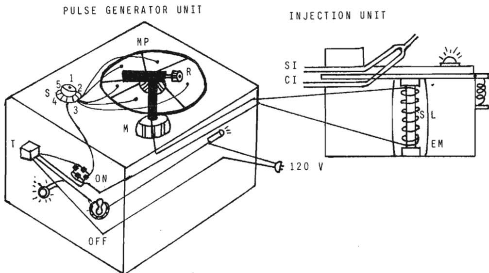
Fig. 2 Schematic drawing of the pulse generation and injection units. T, transformer; S, switch; MP, metal plate; R, rotor; M, rotor motor unit; SI, sample introduction; CI, carrier stream; SL, solenoid; EM, electromagnet
