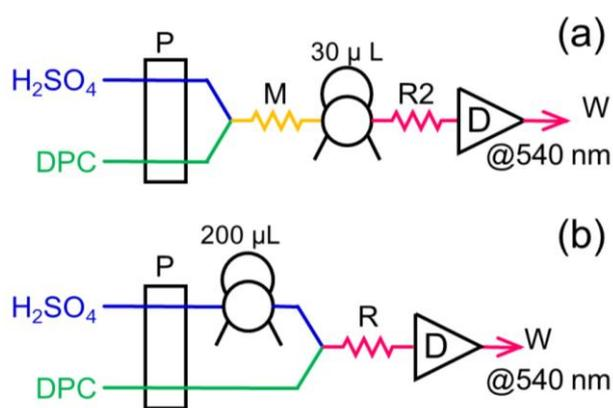
Fig. 1 Flow injection analysis (FIA) systems for chromium determination. (a) First FIA system reported for chromium [18], and (b) two-line FIA system in JIS K0170 6.3.3. P = pump, M = mixing coil, I = injector, R = reaction coil, D = detector, and W = waste
