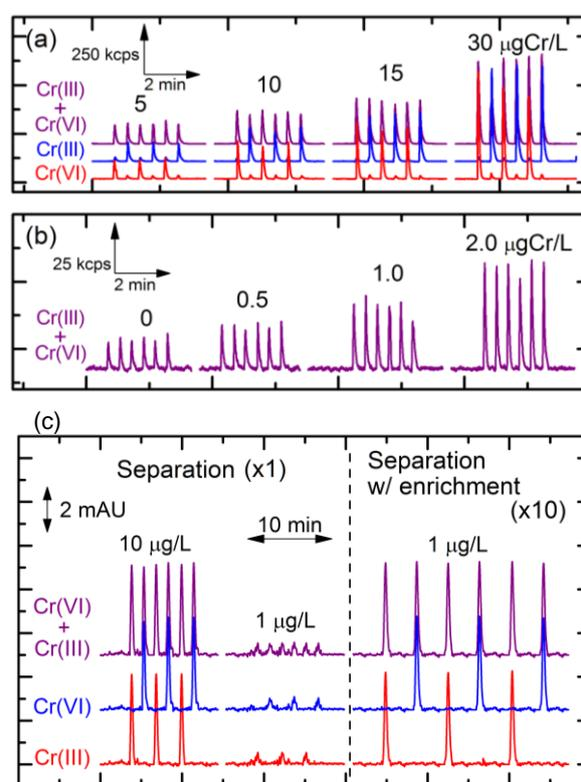
Fig. 4 Response chart obtained with (a, b) inductively coupled plasma mass spectrometry and (c) a diphenylcarbazide-based flow injection analysis system with sample/acceptor flow rate based in-line preconcentration.
