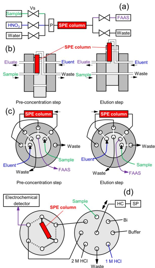
Fig. 2 Solid phase column integrated flow injection analysis (FIA) system with the column integrated in (a) a conventional FIA [40], (b) an injector [41], (c) a five-port valve [42], and (d) a sequential injection analysis (SIA) system [43].
