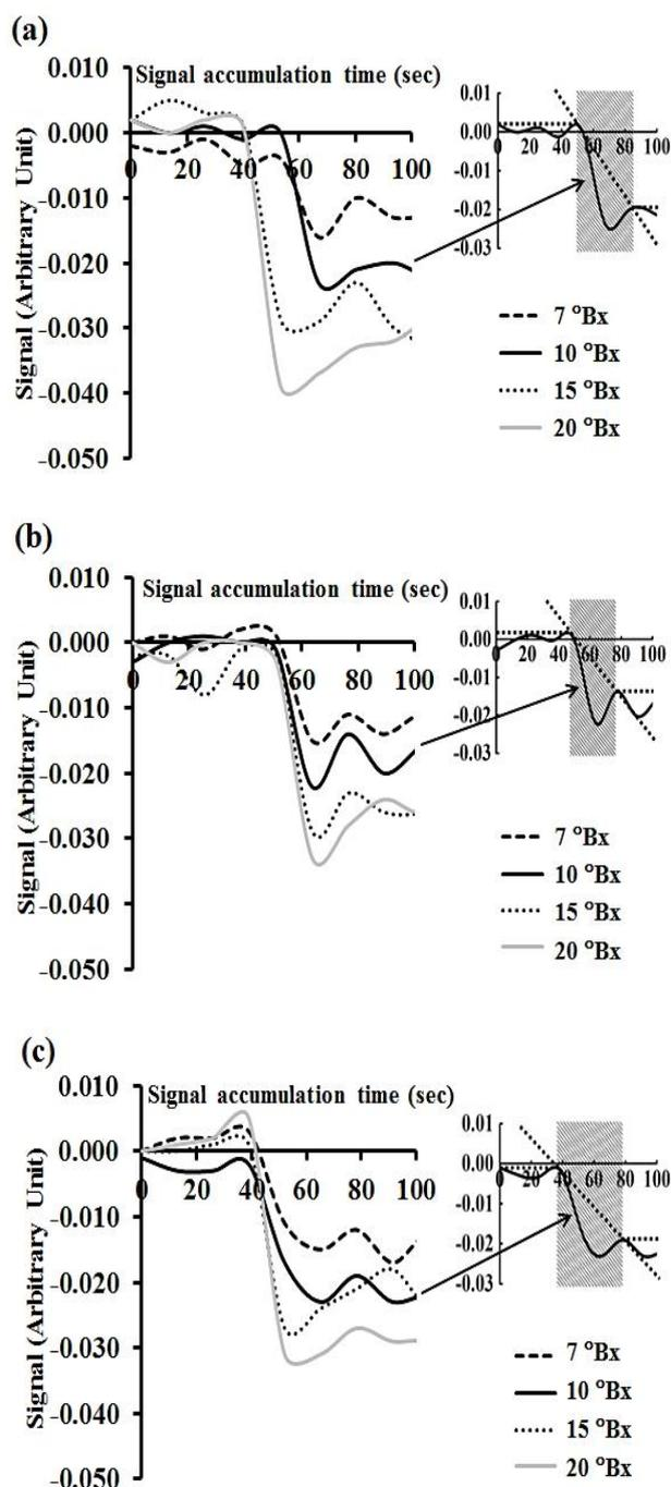
Figure 3. Response signals from standard sucrose solutions (7-20 °Bx) obtained at 700 nm, with data acquisition frequency of 1 point per sec, using various chip angles (a) 60°, (b) 65°, and (c) 70 degrees. The inset shows an example of peak integration of the light scattering signal due to 10 °Bx solution.
