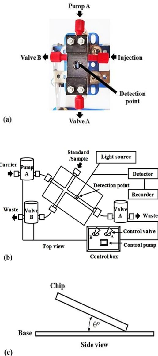
Figure 1. (a) Components of the simple LOC, (b) the diagram of the overall system showing the LOC connected to pumps, valves and a control box, and (c) the side view diagram showing the angle of the LOC with respect to the horizontal plane.
