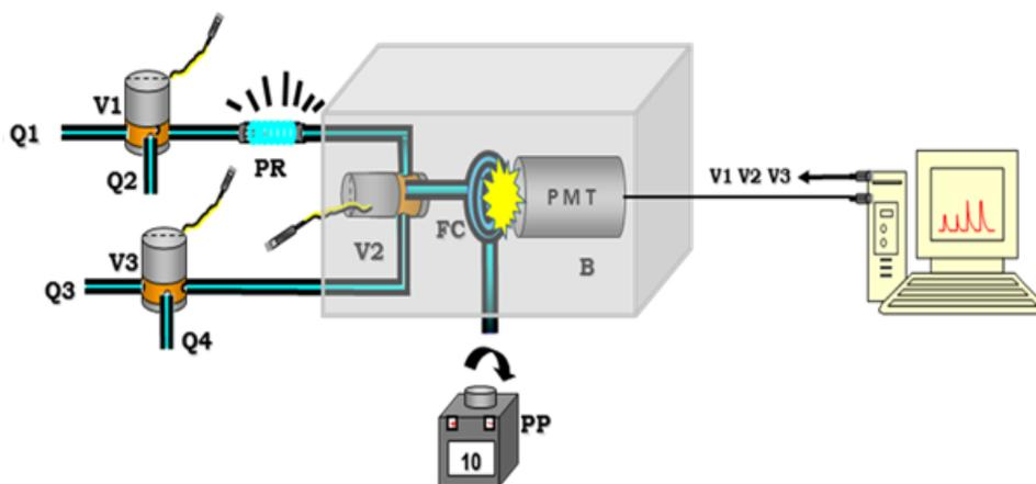
Fig. 2 Solenoid valve flow-assembly for determination of imidazolinones.
