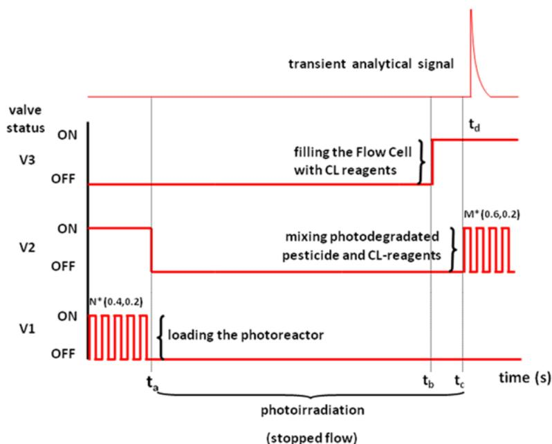
Fig. 3 Schematic profile of a multi-insertion cycle.  $N^*(t_1, t_2)$ .  $N$ : number of insertions. In each insertion the solenoid valve is  $t_1$  seconds ON and  $t_2$  seconds OFF.
