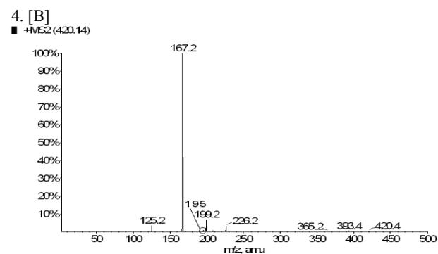
Figure 4. [A and B] Product ion mass spectrum of cypermethrin and fenvalerate respectively
