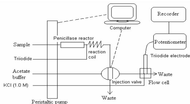
Fig. 1 FIA set-up used in the studies.
