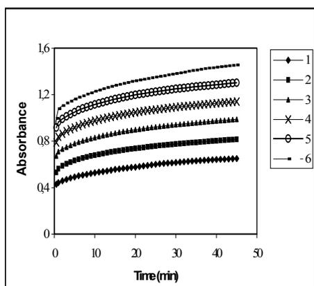
Figure 10. Absorbance vs. times curves for the reaction between FMT and  $\text{KMnO}_4$ :  $\text{KMnO}_4$   $2.5 \times 10^{-3} \text{ mol L}^{-1}$  and FMT (1)  $5.93 \times 10^{-6} \text{ mol L}^{-1}$ ; (2)  $1.18 \times 10^{-5} \text{ mol L}^{-1}$ ; (3)  $1.78 \times 10^{-5} \text{ mol L}^{-1}$ ; (4)  $2.37 \times 10^{-5} \text{ mol L}^{-1}$ ; (5)  $2.96 \times 10^{-5} \text{ mol L}^{-1}$ ; (6)  $3.56 \times 10^{-5} \text{ mol L}^{-1}$ .
