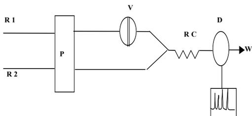
Figure 1. Flow injection system used for determination of FMT. R1: sodium hydroxide, R2: potassium permanganate, P: pump, V: injection valve, RC: reactor coil, D: detector, W: waste.
