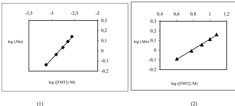
Figure 9. Limiting logarithmic plot for molar ratio of reaction  $\text{KMnO}_4$  / FMT: (1) log Absorbance vs. log  $[\text{KMnO}_4]$ ; (2) log Absorbance vs. log  $[\text{FMT}]$ .
