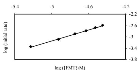
Figure 11. log rate (dA/dt) of the reaction between FMT and  $\text{KMnO}_4$  vs. log FMT concentration
