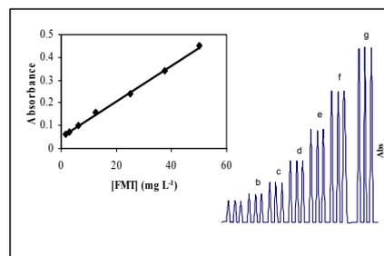
Figure 8. Typical spectrophotometric response of FMT with permanganate solution using the optimum FI operating conditions : (a) 1.5  $\text{mg L}^{-1}$ , (b) 3.1  $\text{mg L}^{-1}$ , (c) 6.2  $\text{mg L}^{-1}$ , (d) 12.5  $\text{mg L}^{-1}$ , (e) 25  $\text{mg L}^{-1}$ , (f) 37.5  $\text{mg L}^{-1}$ , (g) 50  $\text{mg L}^{-1}$
