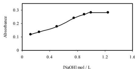
Figure 3. Effect of sodium hydroxide concentration on the absorbance of FMT. KMnO<sub>4</sub> =  $2.5 \times 10^{-3}$  M, flow rate = 2 mL/min, reactor length = 1.4 m and injection volume = 100 µL
