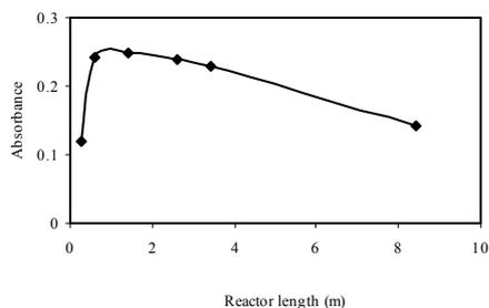
Figure 6. Effect of reactor length on the absorbance of FMT.  $\text{NaOH} = 1.0 \text{ M}$ ,  $\text{KMnO}_4 = 2.5 \times 10^{-3} \text{ M}$ , flow rate = 1.7 mL/min, and injection volume = 135  $\mu\text{L}$ .
