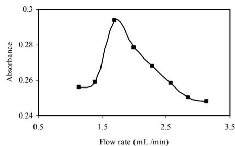
Figure 4. Effect of stream flow rates on the absorbance of FMT. NaOH = 1.0 M, KMnO<sub>4</sub> =  $2.5 \times 10^{-3}$  M, reactor length = 1.4 m and injection volume = 100 µL
