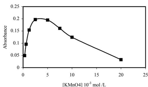
Figure 2. Effect of potassium permanganate concentration on the absorbance of FMT. NaOH = 0.5 M, overall flow rate = 2 mL/min, reactor length = 1.4 m and injection volume = 100 µ
