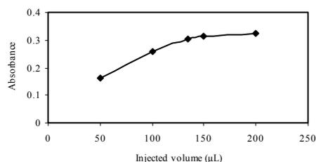
Figure 5. Effect of injected volume on the absorbance of FMT.  $\text{NaOH} = 1.0 \text{ M}$ ,  $\text{KMnO}_4 = 2.5 \times 10^{-3} \text{ M}$ , flow rate = 1.7 mL/min, reactor length = 1.4 m
