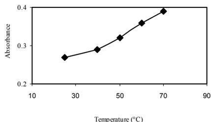
Figure 7. Effect of temperature on the absorbance of FMT.  $\text{NaOH} = 1.0 \text{ M}$ ,  $\text{KMnO}_4 = 2.5 \times 10^{-3} \text{ M}$ , flow rate = 1.7 mL/min, and injection volume = 135  $\mu\text{L}$ , reactor length = 0.6 m.
