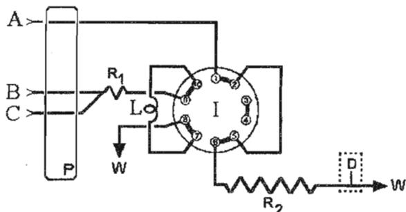
**Fig. 1 Configuration of the miniaturised flow System II** PFTE tubing 0.25-mm i.d.; quartz flow cell of 8- $\mu$ l, 1.00-cm optical path length; A: 1% w/v DPC in 0.4 M nitric acid; B: sample; C: nitric acid for on-line sample conditioning. cm; R<sub>1</sub>: 20 cm; R<sub>2</sub>: 150 cm.
