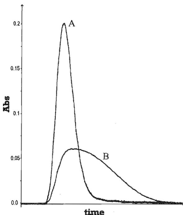
**Fig. 3 Comparison of peak profiles for cobalt sulphate solutions.** A: Miniature System II (tubing radii of 0.25mm i.d., flow cell of 8- $\mu\text{l}$ ); B: Conventional system I (tubing radii of 0.80-mm i.d., flow cell of 80- $\mu\text{l}$ ). (System variables have been chosen in order to obtain the same residence time for both systems).
