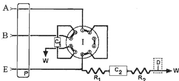
**Fig. 2 Configuration of pre-concentration System IV** PFTE tubing 0.80 mm. id; quartz flow cell of 80- $\mu$ l, 1.00-cm optical path length; E: nitric acid solution; B: sample; A: ammonia solution; C<sub>1</sub>: acid alumina column 70-200 mesh, 1.00-cm x 0.15-cm i.d.; C<sub>2</sub>: DPC-silica column 2.5% w/w, 4.00-cm x 0.15-cm i.d.; R<sub>1</sub>: 60 cm; R<sub>2</sub>: 30 cm.
