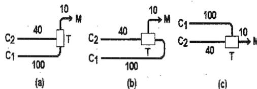
Fig. 1 Three mixing modes of the T-piece.
