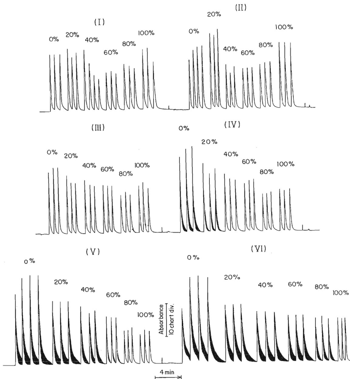
Fig. 4 Recorded graphs for the rhodamine B system in confluence configuration.
