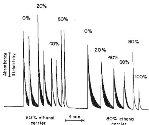
Fig. 7 Smaller sample volume influence in single line FIA manifold.
