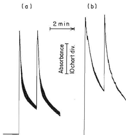
Fig. 8 Effect of pulse damper in single line manifold.
