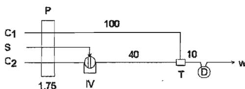
Fig. 2 Flow diagram in confluence configuration. S is the sample solution of rhodamine B,  $C_1$  and  $C_2$  are the carriers, P is the peristaltic pump with indication of the flow rate in  $\text{ml min}^{-1}$ , IV is the rotary injection valve, T is the T-piece, D is the spectrophotometric detection at 553 nm, and W denotes waste. The numbers above the lines represent the tube length in cm.
