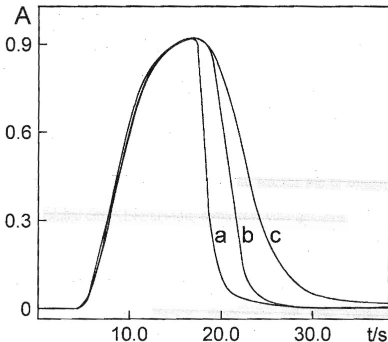
Fig. 2. Transient signals for 1.0 mg L<sup>-1</sup> nitrite: (a) by relocating the coiled reactor after signal maximum; (b) with an intermittent flow rate of 6.2 ml min<sup>-1</sup> introduced immediately before the flow cell, after attaining the maximum signal; and (c) with the system shown in Fig. 1, without relocating the coiled reactor. Results for a 200- $\mu$ l flow cell and 200-cm sample loop.
