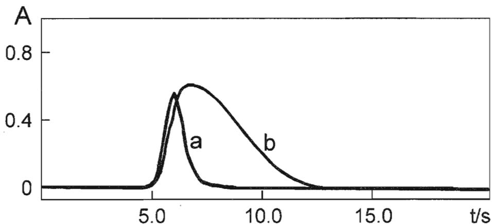
Fig. 4. Transient signals obtained for whole milk powder suspensions: (a) by relocating the coiled reactor after signal maximum and (b) without relocation.
