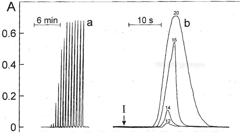
Fig. 3. Transient signals for calcium by flame atomic absorption spectrophotometry. (a) results obtained by relocating the coiled reactor at different times after sample injection (time intervals varied from 11 to 23 s in 1s increments). (b) Overlaid signals obtained by relocating the coiled reactor at 12, 14, 15 or 20 s after injection (I).
