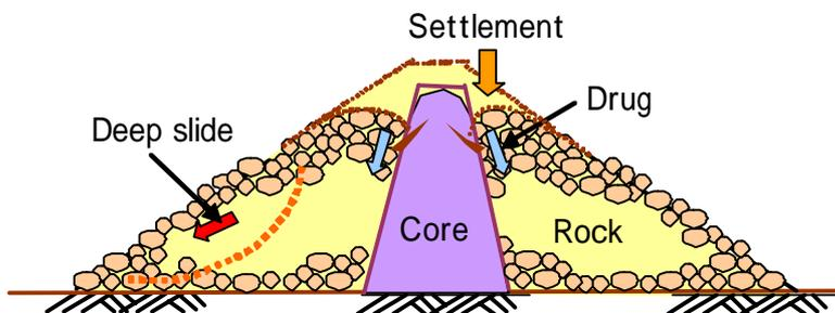
(c) Centrally Located Core Type Rockfill Dam
