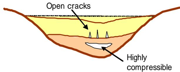
(c) Existence of relatively rigid structure causes inner open cracks due to differential settlement and deformation, especially during earthquake
