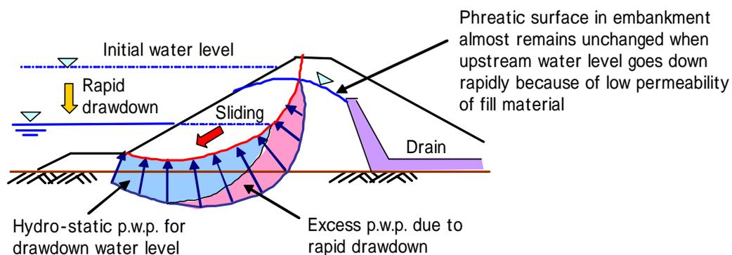
**Fig.2.3 Excess Pore-Water Pressure due to Rapid Drawdown**
