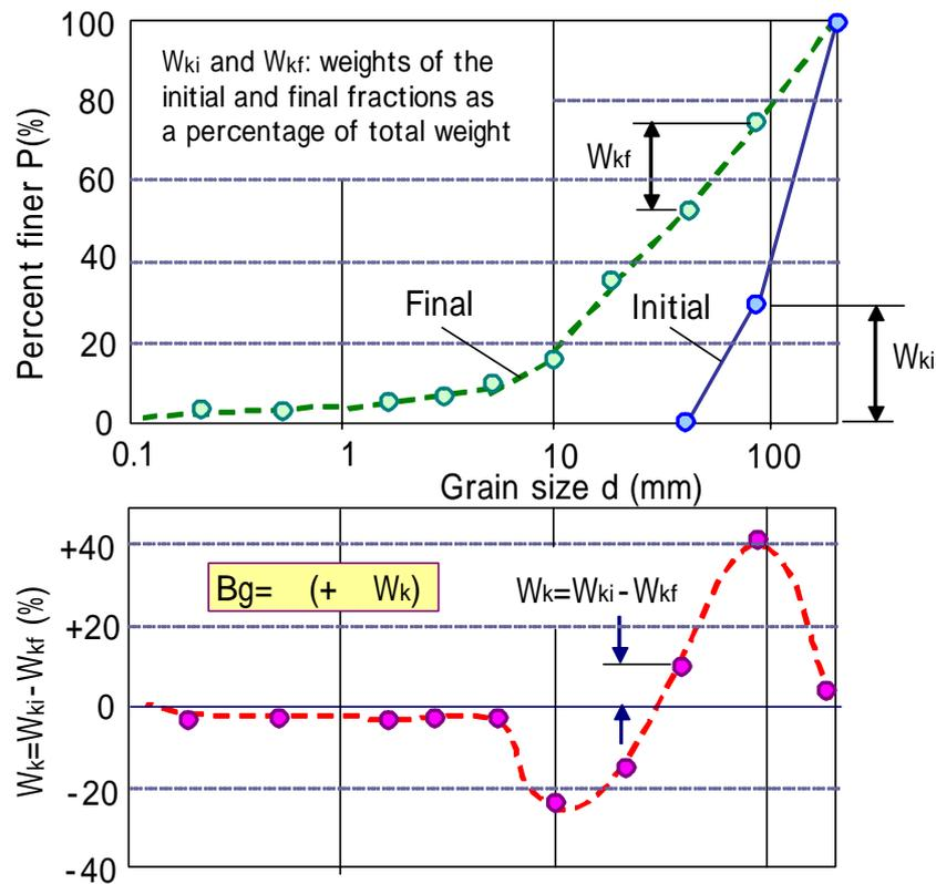
Fig.4.7 Definition of grain breakage  $B_g$
