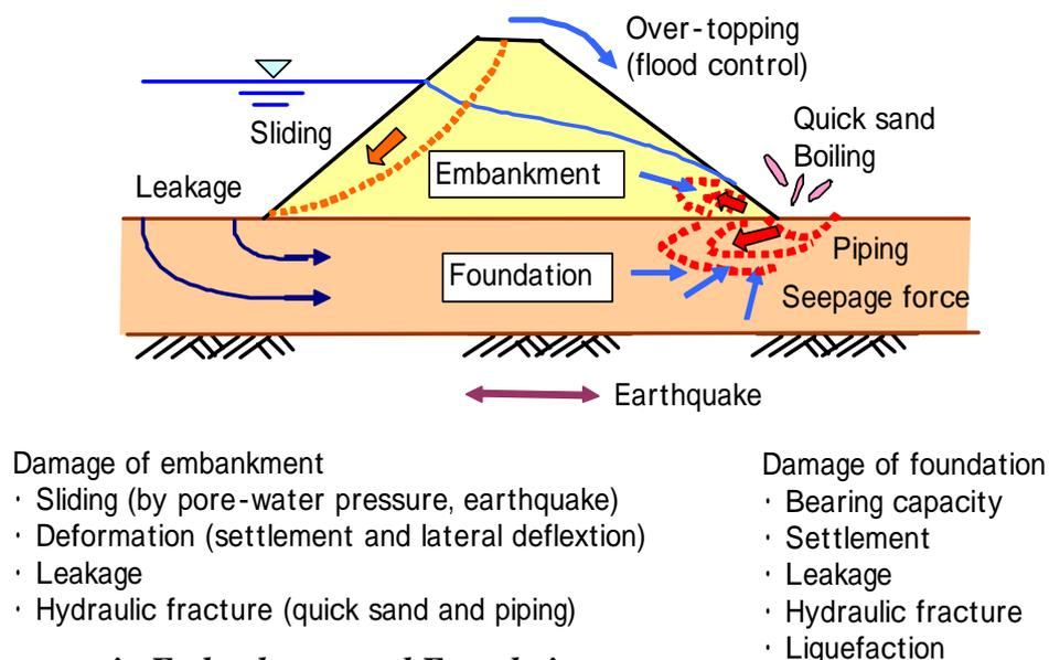
**Fig.2.1 Damages in Embankment and Foundation**
