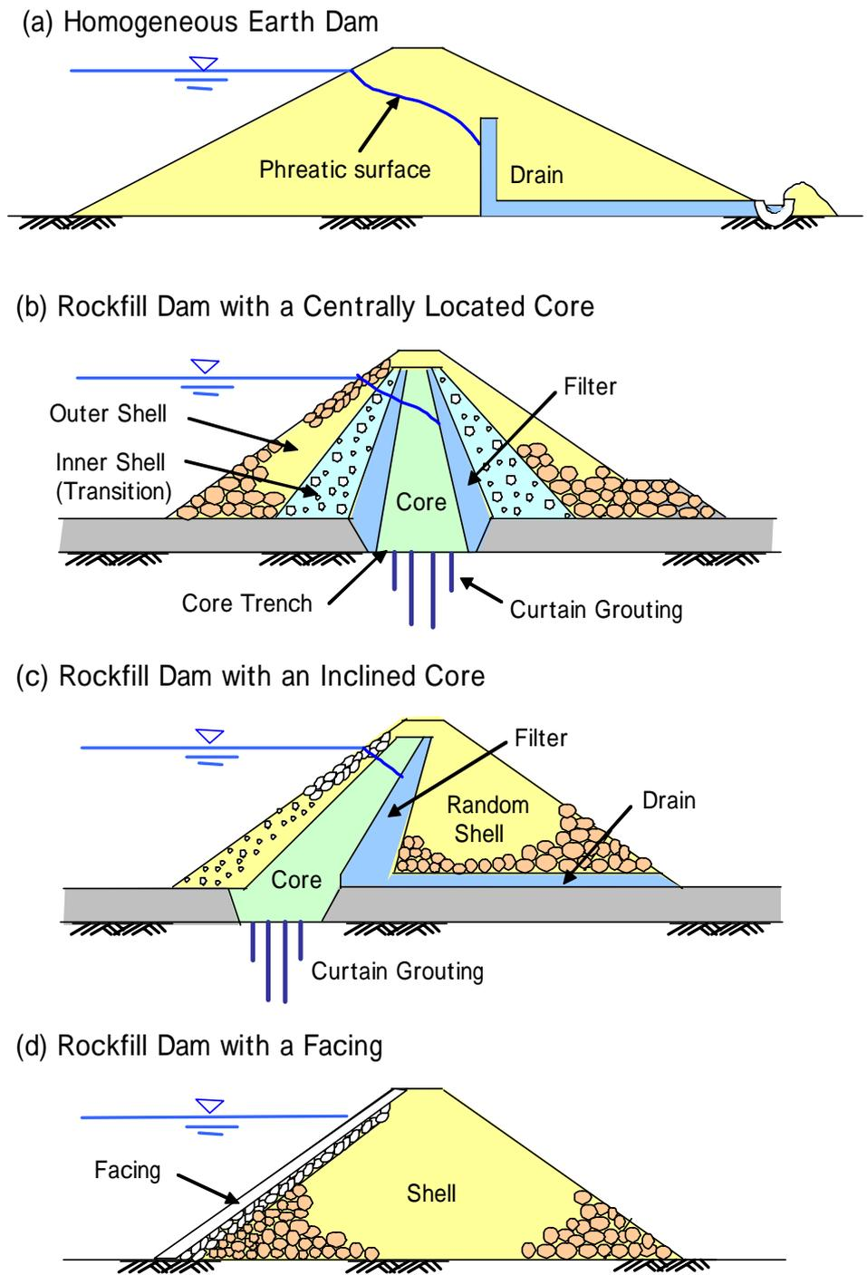
**Fig.1.1 Earth and Rockfill Dams**
