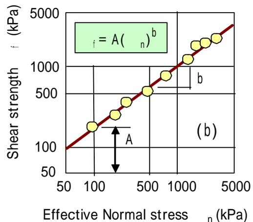
**Fig.3.3 Shear Strength of Non-cohesive Rock Materials**
