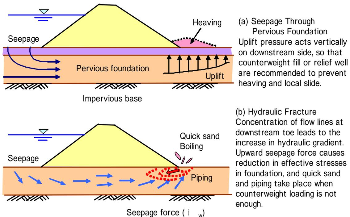
**Fig.2.4 Seepage Through Foundation and Hydraulic Fracturing**
