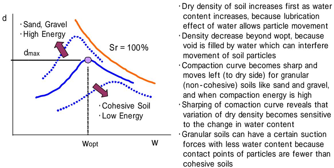
Fig.4.2 General Characteristics of Compaction Curves
