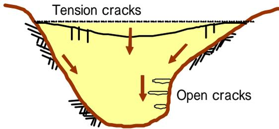
(b) Existence of highly compressible layer of soil in foundation causes local settlement in the embankment, and inner open cracks between them
