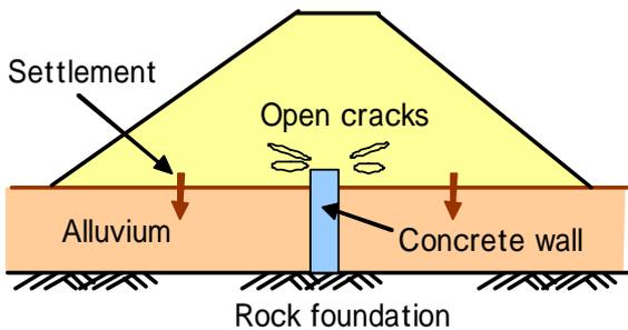
(d) In a narrow central core, arching may take place in core zone which causes low confining stress and open cracks
