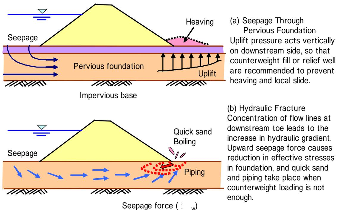
**Fig.2.4 Seepage Through Foundation and Hydraulic Fracturing**
