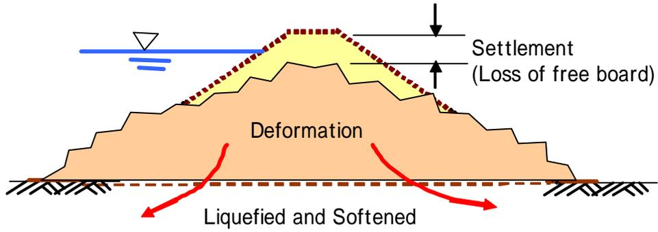
**Fig.2.6 Embankment Failure due to Liquefaction of Foundation**
