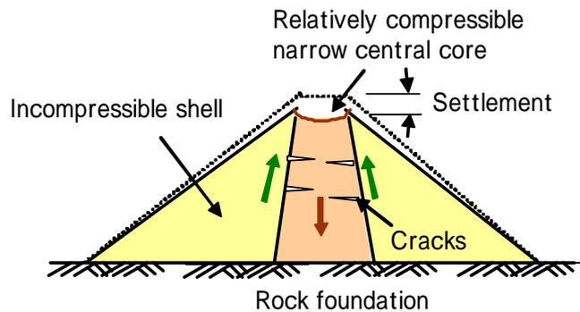
**Fig.2.5 Differential Settlement and Cracking**
