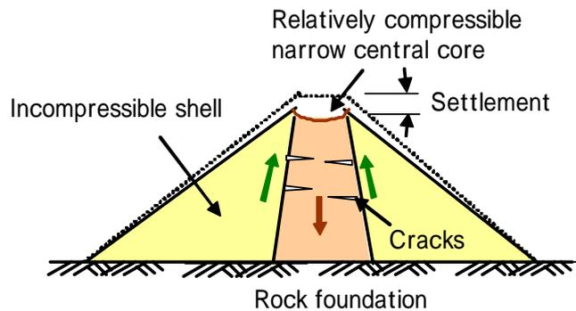
**Fig.2.5 Differential Settlement and Cracking**
