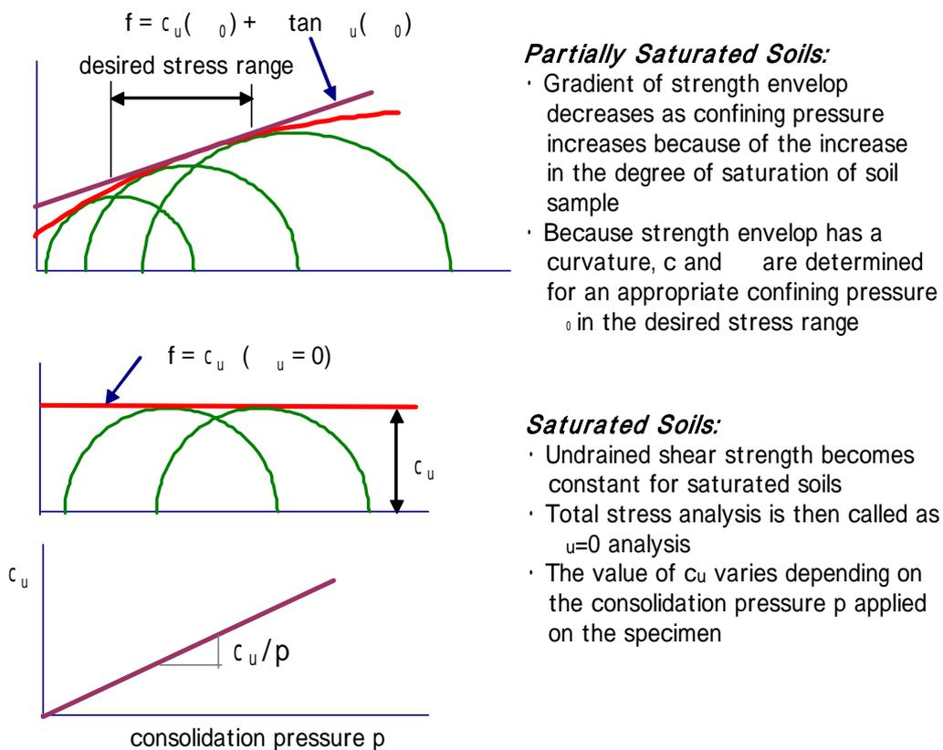
**Fig.3.1 Shear Strength in Total Stress Analysis**
