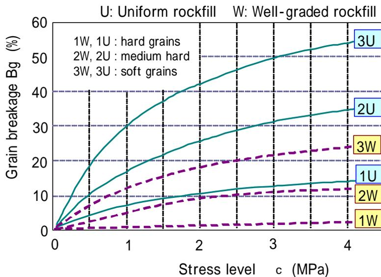
Fig.4.8 relation between  $B_g$ -index and hardness of rockfi
