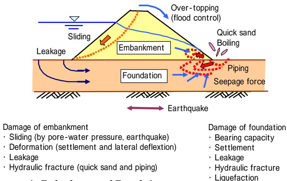
**Fig.2.1 Damages in Embankment and Foundation**
