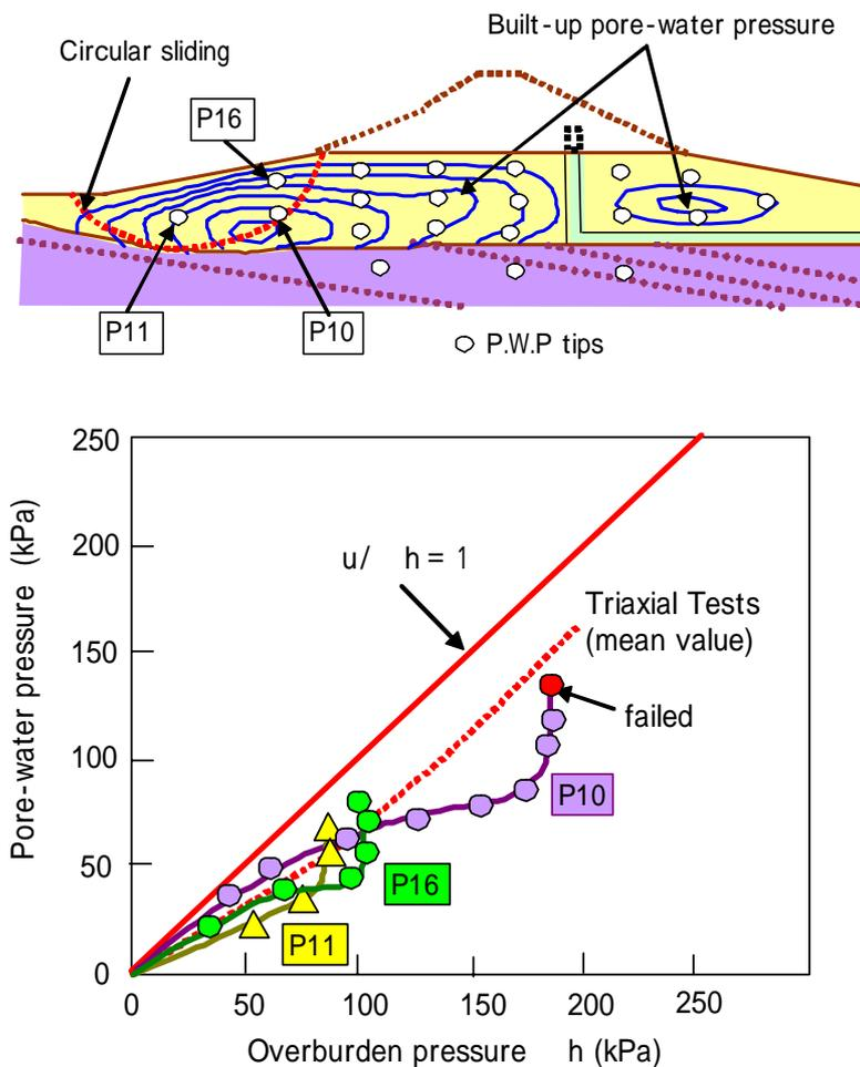
**Fig.2.2 Sliding Failure During Construction**
