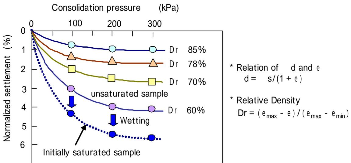
Fig.4.3 Compressibility of Compacted Soils
