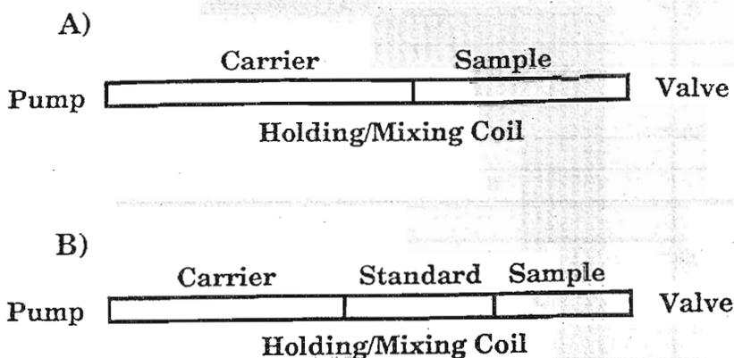
**Figure 3.** Representation of zones present in the holding/mixing coil just prior to injection cycle, for the sequential manifold Fig. 1C, using a A) single and B) dual zone method.
