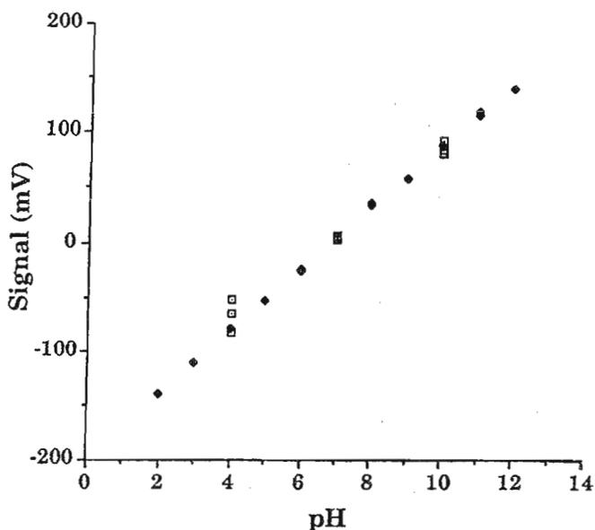
**Figure 6.** Calibration curve for electrochemical pH measurements with the Lazar flat glass combination electrode and dual zone injections by sequential injection methodology. Calibration sample set shown as open squares and sample set as solid diamonds.
