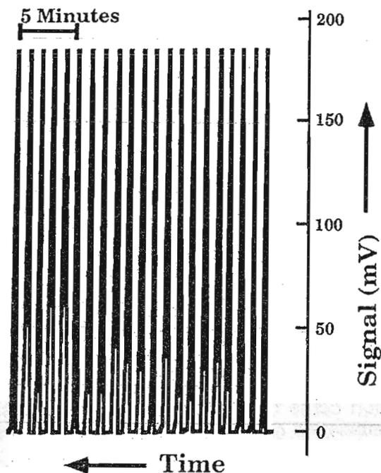
Figure 5. Replicate injections of pH 9 buffer using single zone sequential injection methodology to determine precision. (n=21)
