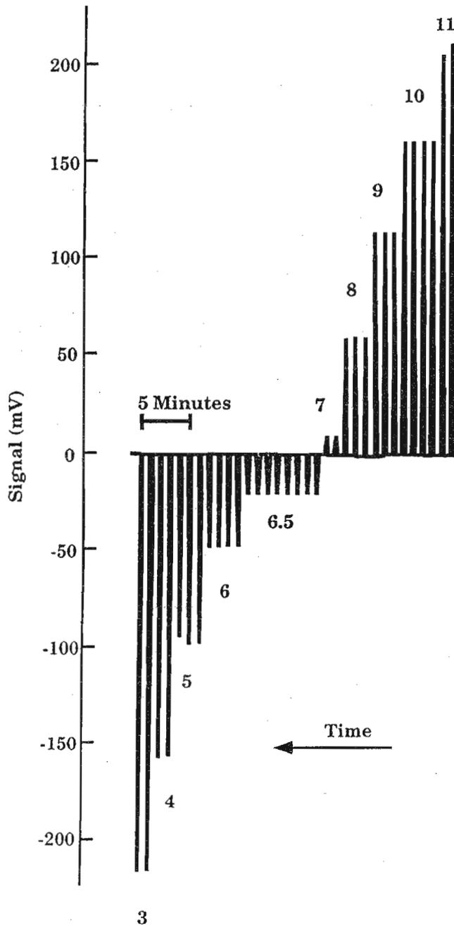
**Figure 4.** Replicate injections of various buffer standards using single zone sequential injection methodology. The electrode responses are shown with a baseline pH of 6.88. The pH values of the buffer standards are shown for each set of injections.
