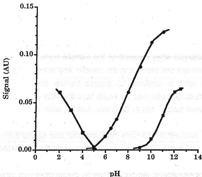
Figure 7. Response curves for the spectroscopic measurements of pH. The three cellulose pads used are shown as: 1) pad 1 sensitive to pH 1-3 (solid squares), 2) pad 2 sensitive to pH 6-9 (solid circles), and 3) pad 3 sensitive to pH 9-12 (solid diamonds). The response observed is consistent with the titration of an acid-base indicator over its sensitive range.
