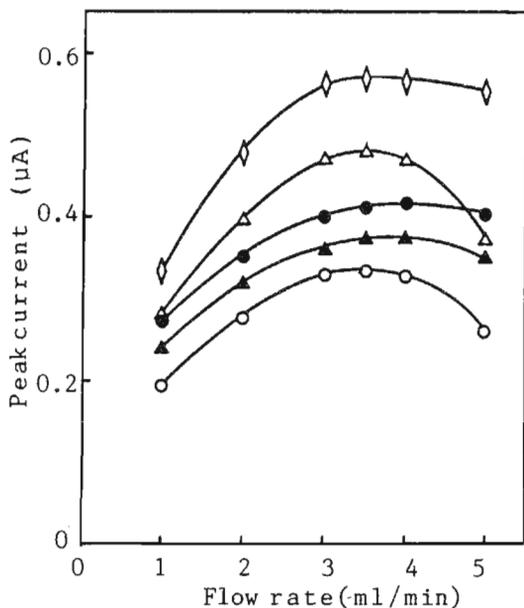
Fig. 3. Effect of flow rate on the peak current. The first peak (○) and second peak (●) were obtained for the injection of a 5- $\mu$ l aliquot of solution containing 100mg/dl cholesterol palmitate and 100mg/dl glucose. Similarly the first peak (△) and second peak (▲) were obtained for control serum (5 $\mu$ l). Only the first peak (◇) was obtained for 100mg/dl cholesterol (5 $\mu$ l). Conditions are described in the text.
