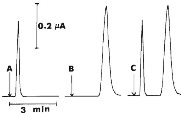
Fig. 2. FIA signals from solutions containing: (A) 100mg/dl cholesterol palmitate; (B) 100mg/dl glucose; (C) 100mg/dl cholesterol palmitate and 100mg/dl glucose.
