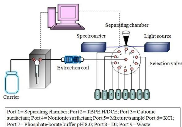
Fig. 1 Schematic diagram of SI-LAV for successive determination of cationic and non-ionic surfactants.
