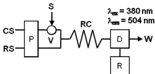
Fig. 1 Flow diagram for the fluorophotometric detection of Al<sup>3+</sup> with 8-quinolinol.
