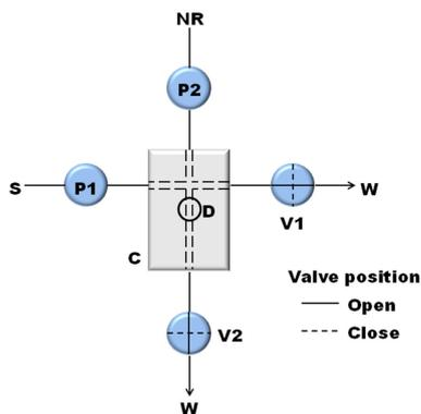
Fig. 1 Schematic diagram of the LOC system
