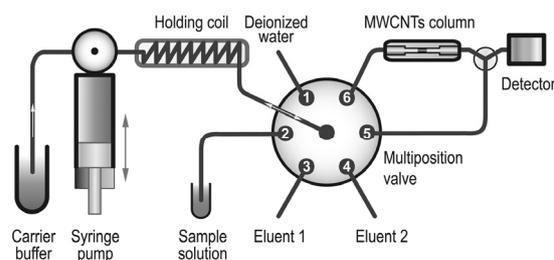
Figure 3. Flow manifold of the sequential injection multiwalled carbon nanotubes (MWCNTs) microcolumn-based solid-phase extraction system for the isolation of basic protein species. [From Ref.38, Z. Du *et al*, Chem. Eur. J., 2007, 13, 9679-9685, by permission of the John Wiley & Sons, Inc.]
