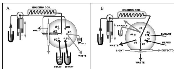
Figure 1. The schematics of  $\mu$ -AC(A) and  $\mu$ -BIS(B) systems. Both  $\mu$ -AC and  $\mu$ -BIS were based on a micro-sequential injection device composed of a syringe pump, a two-way valve, a holding coil, and a lab-on-valve (LOV) manifold mounted on a six-port multi-position valve. [From Ref.21, Y. Gutzman *et al*, Analyst, 2006, 131, 809-815, by permission of the Royal Society of Chemistry]
