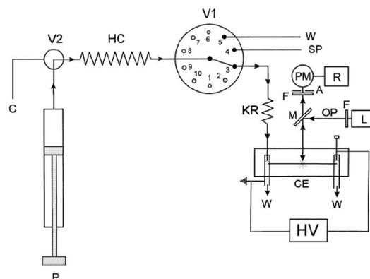
Figure 2. Schematic diagram of the SI-sample introduction microfluidic CE system. [From Ref.28, Q. Fang *et al*, *Anal. Chim. Acta*, 1999, 390, 27-37, by permission of the Elsevier Science Publishers]
