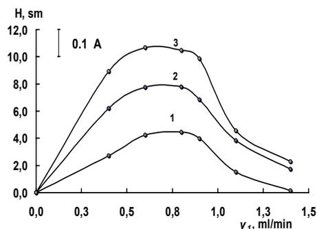
Fig.6. Effect of the carrier flow rate on the peak height H for the following concentration of ALX (mM): 1- 0.10, 2- 0.25, 3- 0.50.
