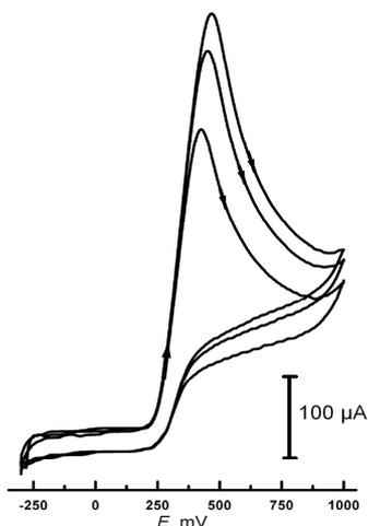
Fig.5. Cyclic voltammograms of a GC electrode (100 mV/s) in the buffered solution of 10.0 mM and 50 mM GSH (pH 7.14).
