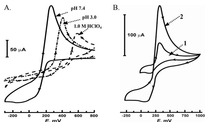
Fig.4. Typical cyclic voltammograms for ALX (A); DUA (B1) and the reaction mixture of ALX and L-cysteine at pH = 7.4 (B2) at a GC electrode. Concentration of ALX and DUA - 5.0 mM, scan rate - 100 mV/s.
