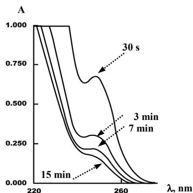
Fig.2. Spectral changes during spontaneous decomposition of 0.1 mM ALX (pH 7.2).
