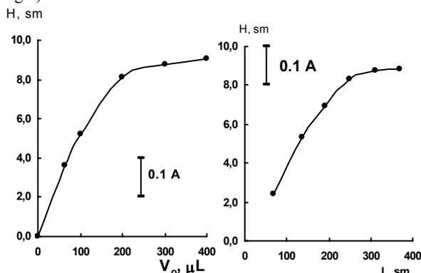
Fig.7. Effects of the sample volume  $V_0$  and the length L of reaction coil on the peak height of ALX.
