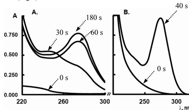
Fig.3. Time-dependent spectral changes during interaction of ALX with L-cysteine (A) and unithiol (B) at 25°C. Reaction mixtures contain 0.1 mM of ALX and 1.0 mM of RSH in a Tris-HCl buffer solution (20 mM, pH 7.2).
