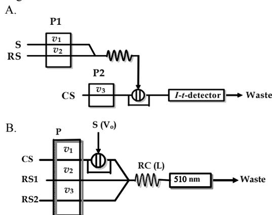
Fig.1. FI manifolds for the determination of ALX with amperometric (A) and spectrophotometric (B) detection.
