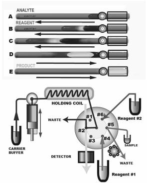
**Fig. 1 (top):** Principle of Sequential Injection. **Fig.1. (bottom):** Configuration of  $\mu$ SI-LOV system. The apparatus comprises a 500  $\mu$ L high-precision, bi-directional syringe pump leading to a 900  $\mu$ L holding coil and the Lab-on-Valve unit mounted atop a 6-port selector valve. The flow cell is contained within the LOV unit with the ends of the fiber optic cables spaced 11mm apart, creating a 22  $\mu$ L flow cell. (Reproduced with permission from ref. 6).
