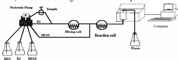
Figure 1: Schematic diagram of the FIA system manifold used for the determination of iron
