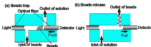
Fig. 2 Jet ring cell for beads injection technique with optical fibers for photometric detection.
