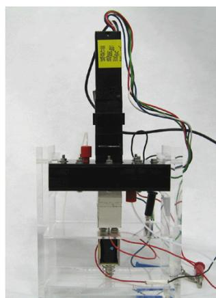
Photo 2 Immunoreaction cell for magnetic microbeads injection technique.
