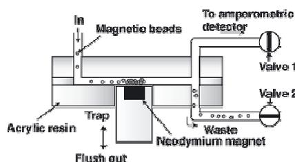
Fig. 6 Schematic flow-through type immunoreaction cell
