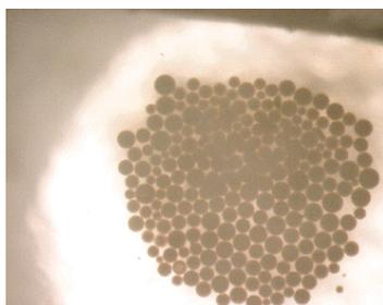
Photo 1 Magnetic microbeads coated with agarose gel.
