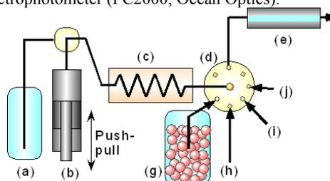
Fig. 1 SIA system combined with beads injection technique.
