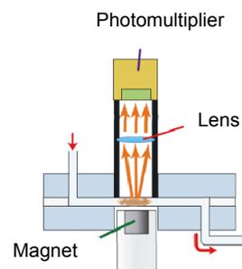
Fig. 3 Immunoreaction cell with magnet and photomultiplier.
