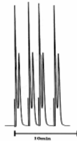
Fig.3 Flow-injection responses for four injections of the the serum sample. Each second peak is L-glutamate. Serum was diluted with 0.05M carbonate buffer (pH9.0) and filtered through an ultrafiltration membrane. The filtrate (10 μL) was injected into the system. [42]
