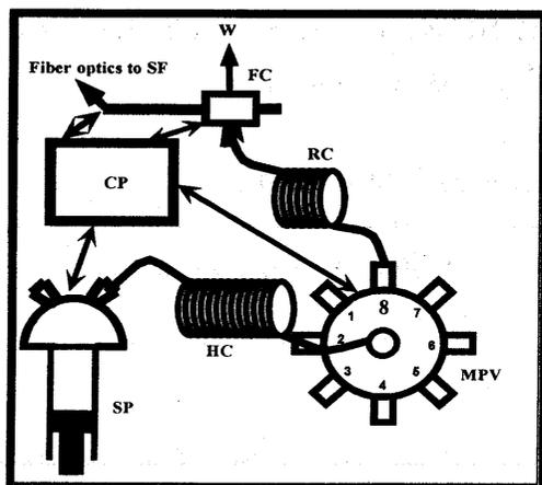
Fig. 1 Schematic diagram of the SI manifold. SP, syringe pump; CP, computer; RC, reaction coil, 45cm length and 0.8 ID; HC, 200 cm holding coil of 0.8 mm ID; MPV, eight ports selector valve; FC, flow through cell placed in fluorimeter compartment; SF, Spectrofluorometer; W, waste.
