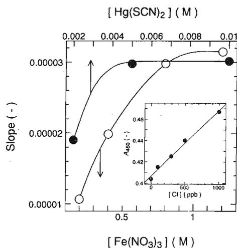
**Figure 3.** The effect of the concentration of iron(III) nitrate and mercury(II) thiocyanate on the slope of the calibration curve. The volumes of the injected zones are 50  $\mu$ L (sample), 10  $\mu$ L (reagent), and 50  $\mu$ L (spacer). Inset: Typical calibration curve of chloride in low concentration region. The volumes of each injected zone are 100  $\mu$ L (sample), 20  $\mu$ L (reagent), and 50  $\mu$ L (spacer). Light pass is 10 mm.
