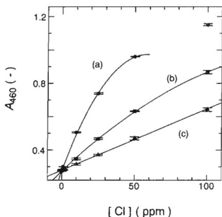
**Figure 4.** The calibration curve of chloride in the high concentration region. The stacked zones used were (a) 100  $\mu\text{L}$  (sample), (b) 20  $\mu\text{L}$  (sample), and (c) 10  $\mu\text{L}$  (sample), 20  $\mu\text{L}$  (reagent), and (a) 50  $\mu\text{L}$  (spacer) and (b) & (c) 100  $\mu\text{L}$  (spacer). Calibration curves obtained were:
