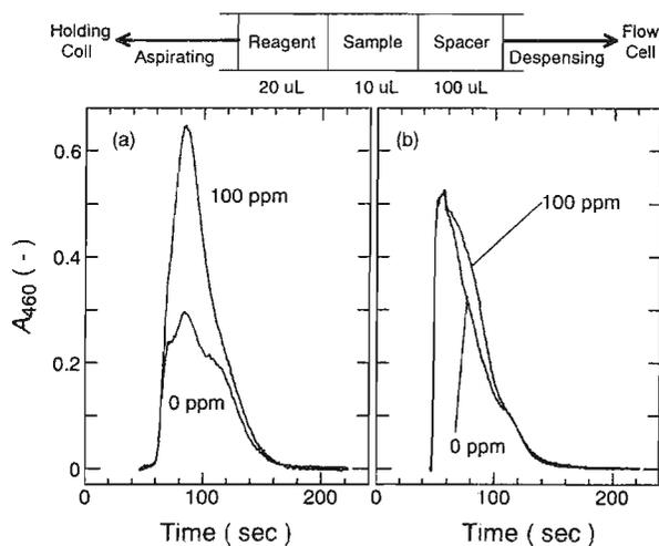
**Figure 2.** The peak shape obtained for the blank control and the 100 ppm sample. The stacked zones of sample, reagent, and spacer are depicted for the chloride assay. Spacer is (a) water or (b) reagent. Light pass and integration time are (a) 5 mm and 500 msec, and (b) 1 mm and 200 msec.
