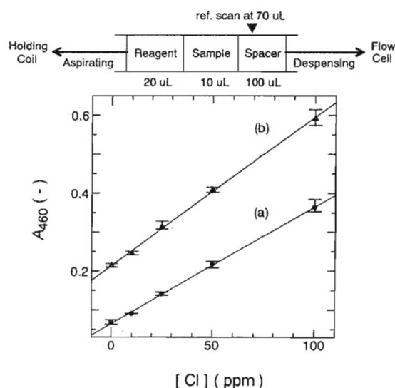
**Figure 5.** The calibration curves based on the reference scan with the spacer. The stacked zones of 10  $\mu\text{L}$  of sample, 20  $\mu\text{L}$  of reagent, and 100  $\mu\text{L}$  of spacer (DI water) are depicted. The dispense rate until reference scan is (a) 3  $\mu\text{L}/\text{sec}$  and (b) 10  $\mu\text{L}/\text{sec}$ , and the delay time for the reaction is (a) 10 sec and (b) 1 sec.
