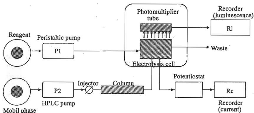
Fig.1 Experimental setup for the ECL-HPLC
